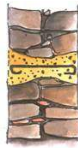
Step 5- The key stone or stitching element
